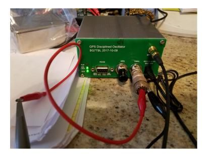
The GPS Discipline Oscillator measures 4 inches by 4 inches. The SMA connector is attached by coax to the GPS antenna. The red alligator clip is feeding a 10 MHz signal to the oscilloscope. 12 VDC powers the unit. Note the green GPS lock LED is lit which indicates the OCXO is receiving GPS time pulses.
